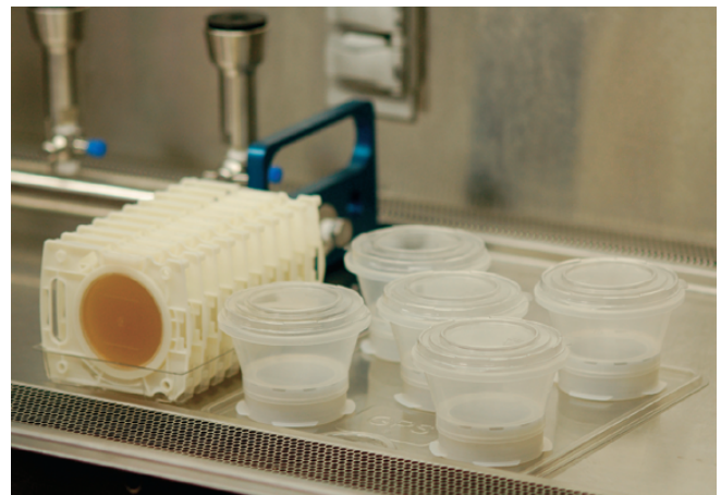
Figure 5 The consumables provided for testing liquid products and raw materials using the Growth Direct system are similar to those used in today's tests. Left: sample cup with membrane filter. Right: growth cassette containing nutrient agar.
