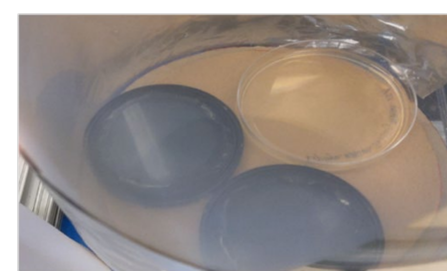
Figure 4. Double Growth Direct® Cassette and a traditional petri plate are placed side-by-side on a rotating base platform for Bioaerosol deposition.
