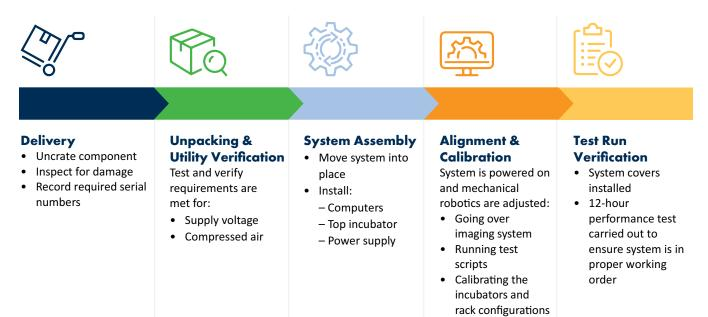
All stages are documented in a comprehensive installation record, ensuring the quality of a thorough installation, safety of the instrument, and continuing with a complete training for our customers.
