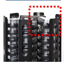
Tip: Ensure that cassettes are stacked flat on top of each other in the carousel. Each carousel has 6 columns that can fit a maximum of 10 cassettes.
