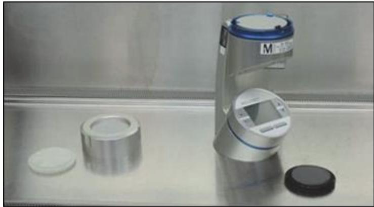
Figure 7-4: Air Samplers and Adapter Clips
