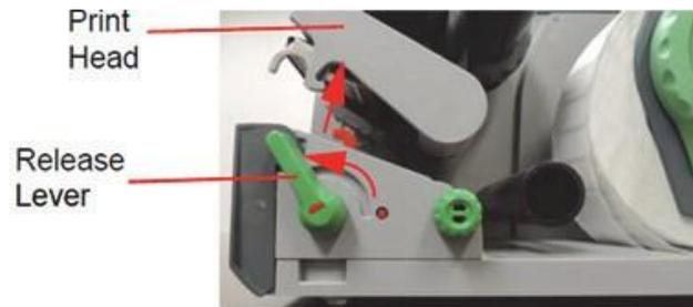
Figure 9-4: Unlocking the Print Head
