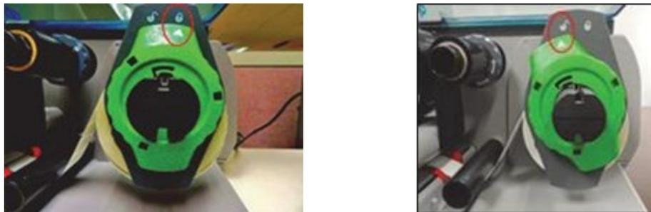
Figure 9-2: Turn the Retainer Ring
