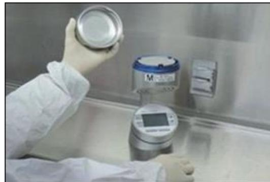
Figure 7-5: Placing the Cassette into the Sampler
