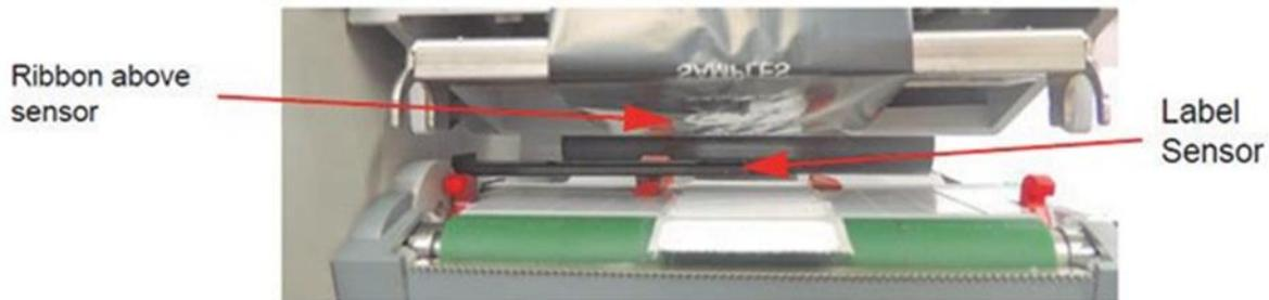
**Figure 9-12: Positioning the Label**
