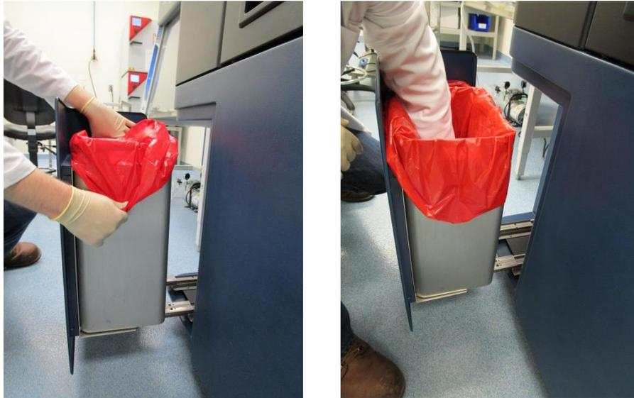
**Figure 3-21: Inserting a New Biohazard Trash Bag**
