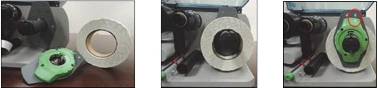
Figure 9-3: Inserting Labels
