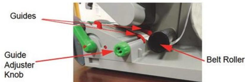
Figure 9-5: Positioning the Label Strip
