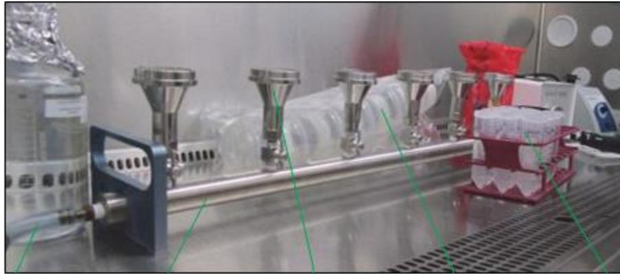
Vacuum tubing      Manifold, 6-Branch      Tulip      Filtration kits      Samples
