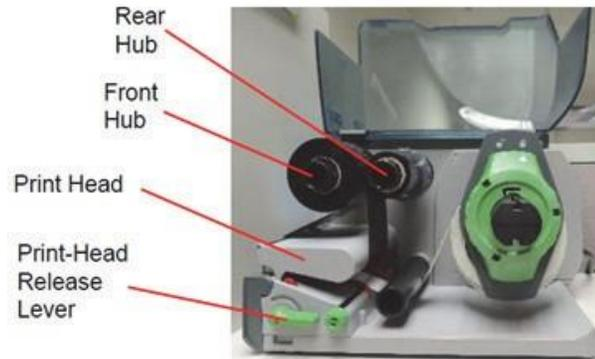
**Figure 9-9: Printer Ribbon Parts**
