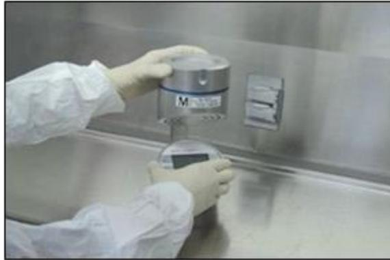
**Figure 7-7: Screwing on the Air Sampler Lid**
