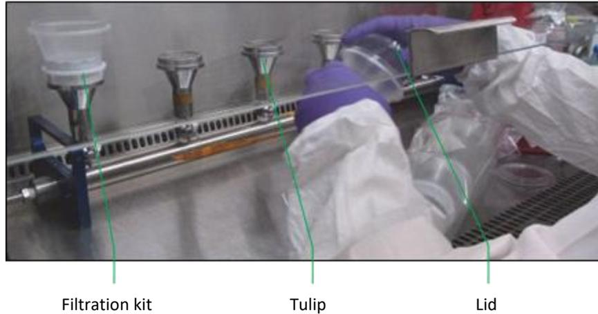
**Figure 6-5: Attach Filtration Kits to Manifold**
