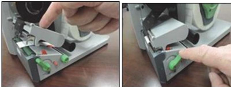
Figure 9-16: Locking the Print Head In Place
