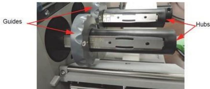
**Figure 9-13: Holding the Hub and Locking the Guide**
