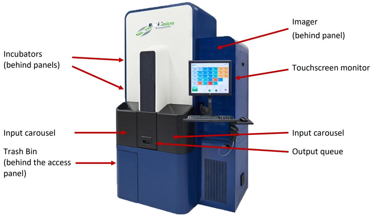
Figure 1-1: Growth Direct® Instrument
