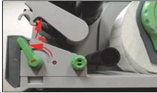
Figure 9-15: Unlocking the Print Head
