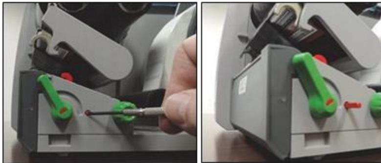
**Figure 9-7: Adjusting the Label Sensor**
