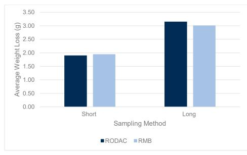
Figure 4. TSA LP80 Media Weight Loss After Active Air Sampling in MAS-100 NT. Cassettes remain in sampler for duration of sampling time.
