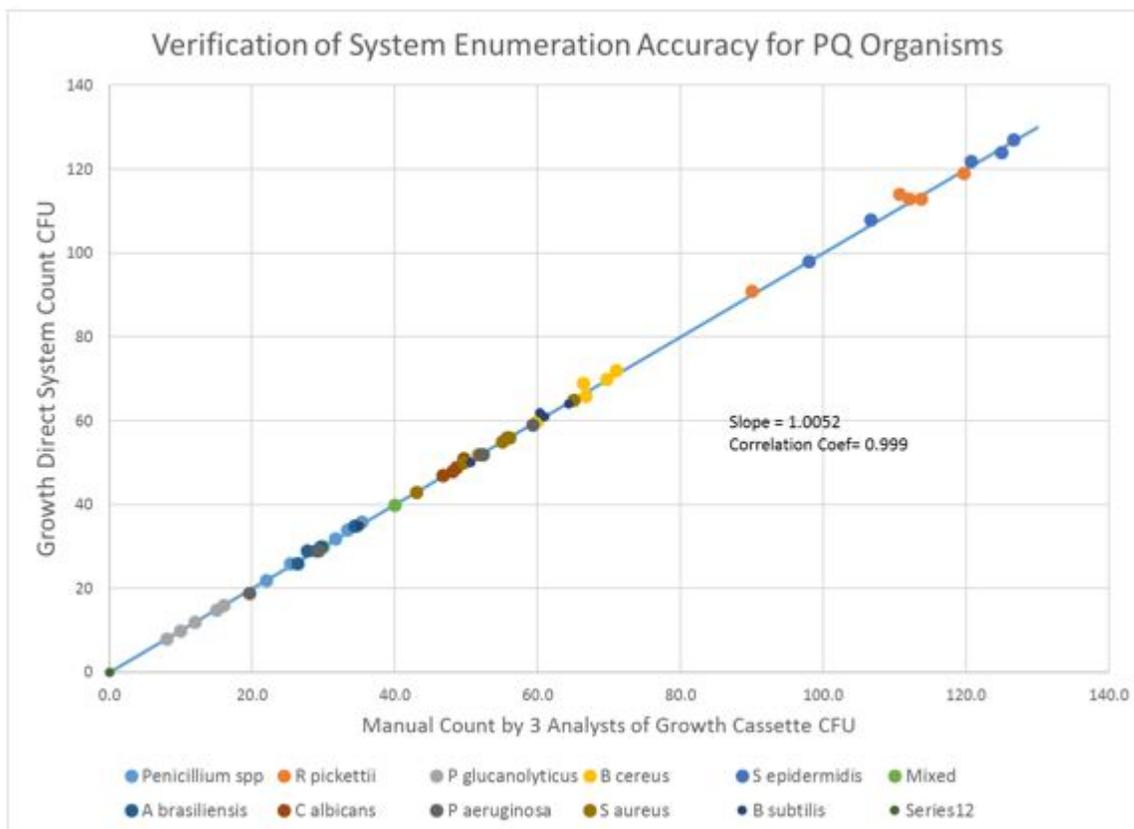
**Fig 1** Correlation of System CFU counts for USP and EM microorganisms compared to the mean CFU count of 3 analysts on the same cassette
